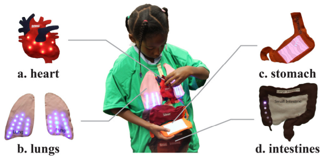
Figure 2. BodyVis shows internal layers of the human body along with physiological phenomena of the wearer. Shown above: (a) the heart vibrates and lights up according to the wearer’s heart rate, (b) the lungs visualize the breathing rate with lights, (c) the stomach shows how food is processed, (d) the intestines illuminate the digestion pathway.
