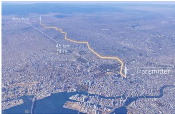
Figure 2: Approximate location of the field trial of the QKD system, with the transmitter in central Tokyo and the receiver towards the western edge of the city. The two locations are connected by an installed telecom fibre pair with a length of 45 km (14.5 dB loss). [Map data: Google, SIO, NOAA, U.S. Navy, NGA, GEBCO, Image Landsat and Japan Hydrographic Association.]
