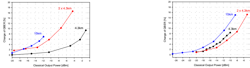
Figure 3: Left: Change of QBER with increasing Output power of a single classical channel for 4.3km (black) 2x4.3km (red) and 15.3km (blue). Right: Change of QBER with increasing Output power of 6 classical channels for 4.3km (black) 2x4.3km (red) and 15.3km (blue).
