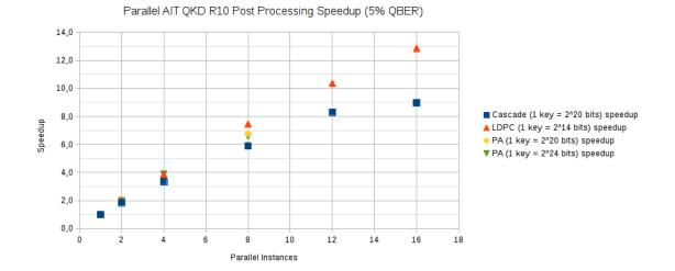
Figure 1: Speedup comparison for parallel instances of some AIT QKD post processing modules
