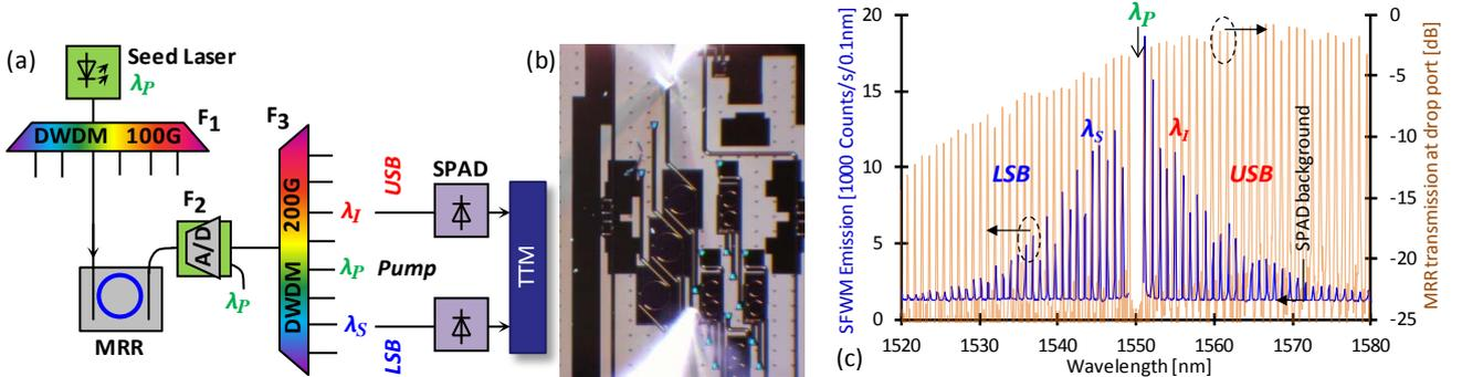
**Fig. 1.** Generation of photon-pairs with photonic integrated silicon micro-ring resonator. (a) Experimental setup, (b) fabricated device, (c) MRR transmission and emission spectra.
