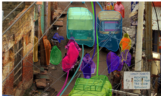
Fig. 1: We highlight the performance of our tracking algorithm, RoadTrack, in this urban video. This frame consists of 27 road-agents, including pedestrians, two-wheel scooters, three-wheel rickshaws, cars, and bicycles. RoadTrack can track agents with 75.8% accuracy at approximately 30 fps on an TitanXp GPU. We observe average improvement of at least 5.2% in MOTA accuracy and 4× in fps over prior methods.
