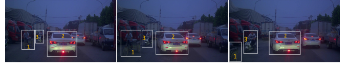
Fig. 3: Qualitative analysis of RoadTrack on the TRAF dataset at night time consisting of cars, 2-wheelers, 3-wheelers, and trucks. Frames are chosen with a gap of 2 seconds ( \sim 60 frames). For visual clarity, each road-agent is associated with a unique ID number. The ID is displayed in orange. Note the consistencies in the ID, for example, the 3-wheeler (1), car (2), and 2-wheeler (3).
