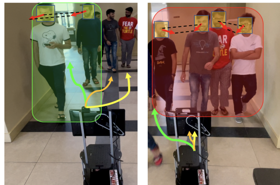
Fig. 1: Our novel navigation method uses our CoMet metric to compute a collision-free trajectory for a robot in real-world scenarios. CoMet identifies groups in crowds and detects intra-group proximity, walking speed, group size and interactions to estimate a group’s cohesion. [Left] In dense scenarios, our navigation algorithm identifies a low-cohesion group (green bounding box) and navigates between its group members (green path) by assuming human cooperation for navigation. [Right] Our method detects a high cohesion group (red bounding box) and plans a trajectory around it. In both cases, other methods such as Frozone [6] (yellow path) and a DRL method [7] (orange path) approach groups with high-cohesion and halt the robot. Overall, our method improves social-compliance and the naturalness of the trajectory.
