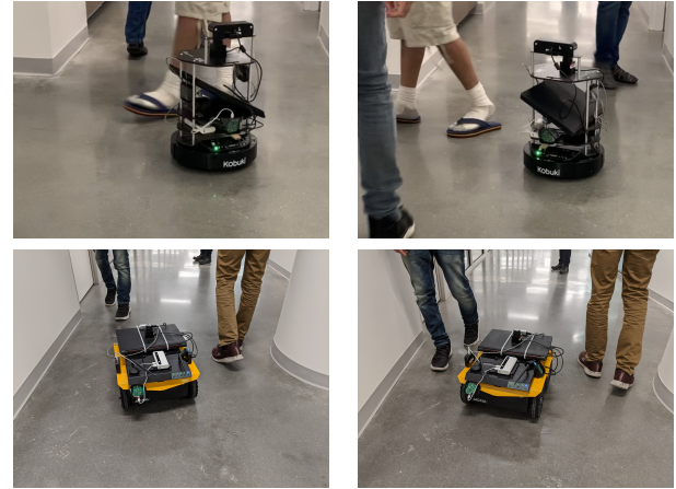
Figure 1: A Turtlebot and Jackal robot using CrowdSteer to navigate in scenarios with pedestrians in a narrow corridor and areas with high occlusion. Our method uses data from multiple sensors such as a 2-D lidar and a depth camera to generate smooth collision avoidance maneuvers. We compare with methods such as DWA[11] and Fan et al[17].
