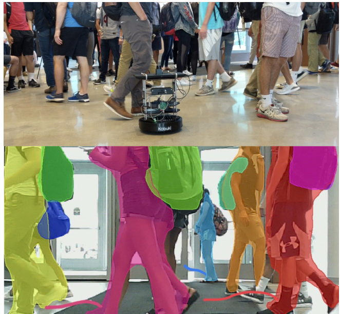
Fig. 1: [Top] Our method implemented on a Turtlebot navigating through a dense crowd. [Bottom] We explicitly track and predict pedestrian motions (marked for the three pedestrians) and use it to train a Deep Reinforcement Learning-based collision avoidance policy. Our network implicitly learns to reduce the occurrence of the freezing robot problem and generates smooth robot trajectories in dense crowds.
