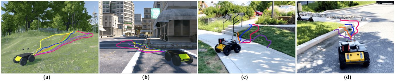
Fig. 5: Robot trajectories when navigating in different simulated and real-world uneven terrains using TERP (pink), TERP w/o attention (yellow), end-to-end Attn-DRL network (violet), ego-graph (orange), Ego-graph+ (green) and DWA (blue). (a) High-elevation; (b) City-curb; (c) real-world medium-elevation; (d) real-world curb. We observe that TERP computes trajectories with low elevation gradients in uneven terrains and is also able to handle challenging curb scenarios well. See [18] for detailed evaluations and results.
