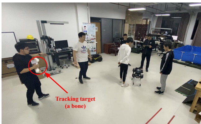
FIGURE 8: The demonstration of the dynamic collision avoidance experiments. We arranged 6 moving pedestrians in this scenarios about 4\text{ m} \times 4\text{ m} in size.
