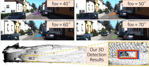
Figure 7: 3D detection results in bird’s eye view with different intrinsic parameters. The red box indicates the ground-truth, and the boxes in other colors indicate our results. Our detection results are very close to the ground-truth in the 3D space, though the visual 2D images are different.
