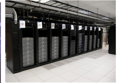
Depththought2: Dell Linux cluster with 9200 cores and 40 nodes with dual GPUs
