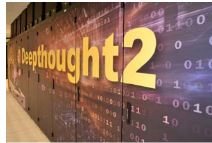
Depththought2: Dell Linux cluster with 9200 cores and 40 nodes with dual GPUs
