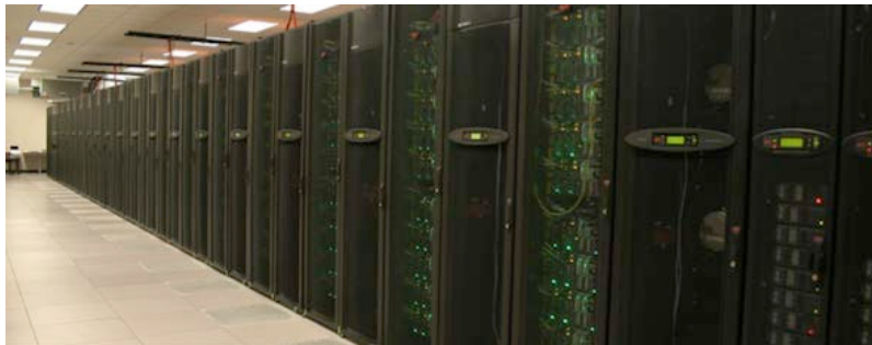
Stampede: Dell Linux cluster with 100,000+ Cores (10 PetaFlops) (All have MIC & some with GPUs)
