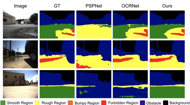
Fig. 4: **Qualitative Results:** Each row highlights the original image, ground truth (GT) label, predictions of two SOTA methods, and prediction of our method. We observe that our method is able to detect different navigable regions and is robust with respect to objects with similar colors.
