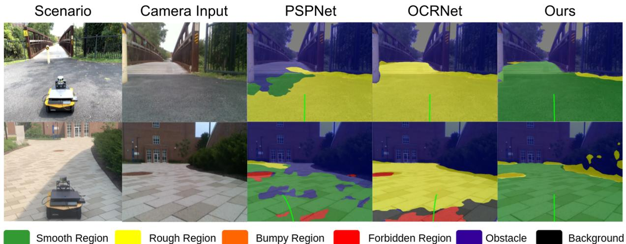
Fig. 3: **Qualitative results in the wild:** We show the real-world performance of GANav and two SOTA methods with pre-trained models on RUGD and RELLIS-3D. The green trajectory is the path of the robot in the next 2 seconds based on its current velocity. While other methods have some false positives for the forbidden region and over-generalize on the rough region (in yellow), our method can correctly identify different regions and stay on the safest path.
