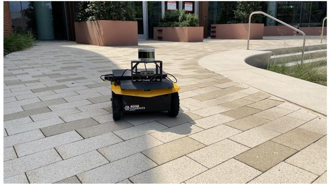
Fig. 5: GANav Setup on a Clearpath Jackal Robot.
