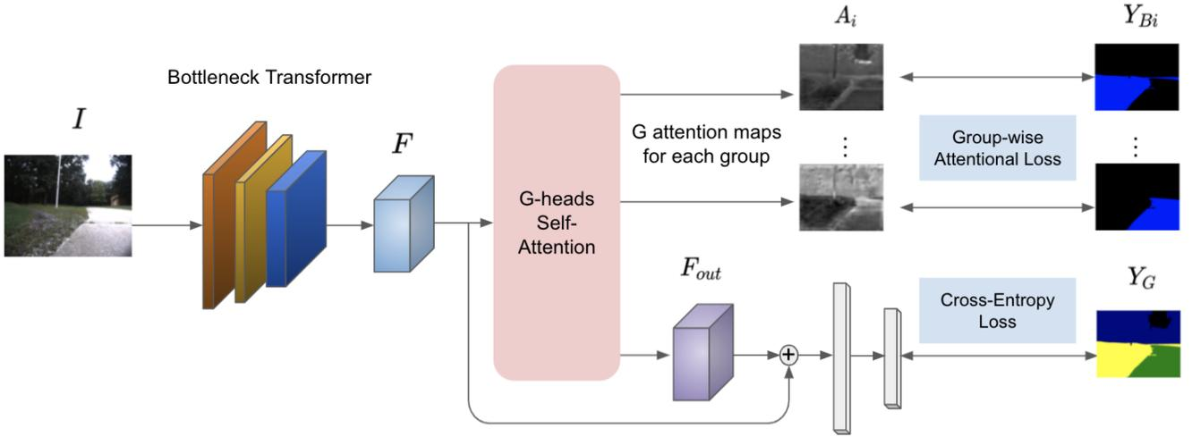
Fig. 2: **Architecture of our proposed network GANav:** We build on the transformer attention backbone [34] and introduce a novel group-wise attention head. The group-wise attention loss acts between the multi-head attention outputs corresponding to each group and the corresponding group-wise binary ground truth to explicitly guide the network towards accurate predictions of different groups.
