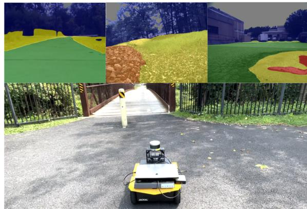
Fig. 1: We highlight the performance of our algorithm on unstructured outdoor terrains. We classify the navigable regions (*top*) using our approach on raw RGB images. The first segmentation result is obtained in the real world from a Clearpath Jackal, while the second and the third are from the RUGD dataset, on which our model achieves an accuracy of 83.24 and an improvement of 6.74–39.1% over prior algorithms.
